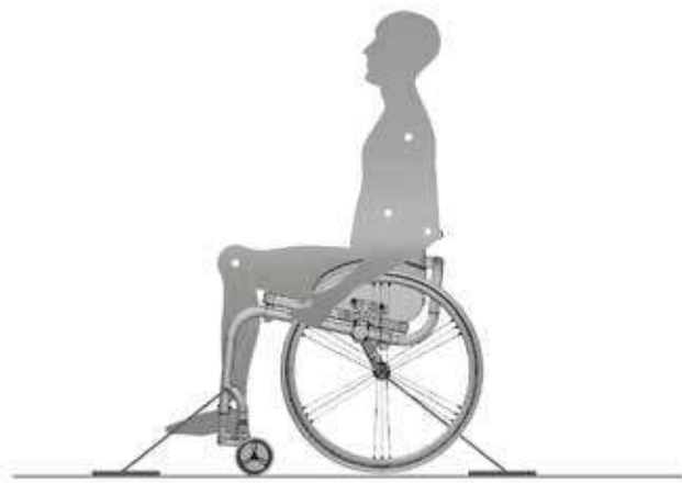
Wheelchair fixing by means of a 4-point securement system
